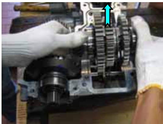
Remove the layshaft
