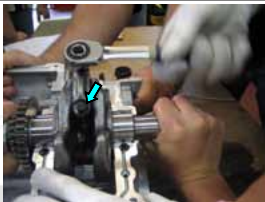
Loosen the connecting rod bolts*2
