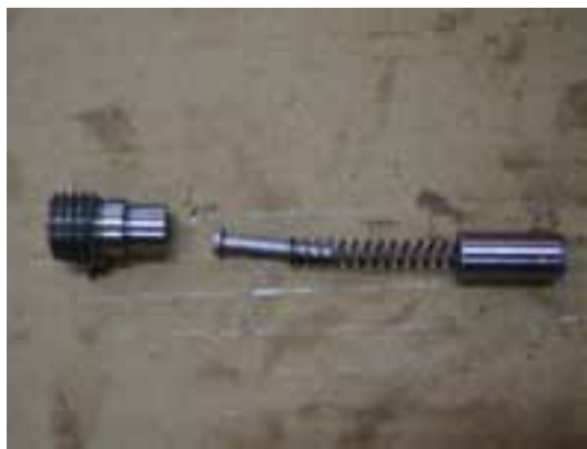
The oil release valve
