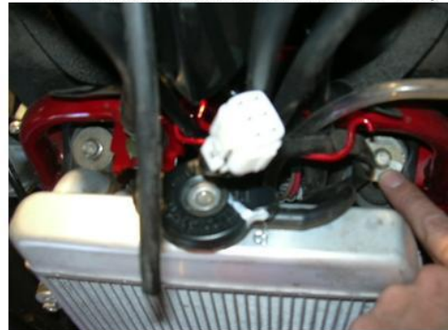
20. Clip removal for fuel line and connections for fuel pump. Take your time, no tools, just hands
