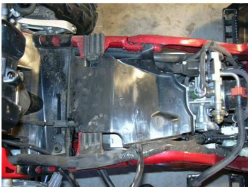
23. The hardest part, heat shield removal
