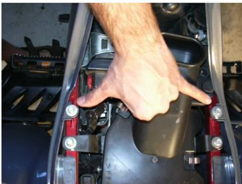
13. Top of gas tank showing connections that need to be removed
