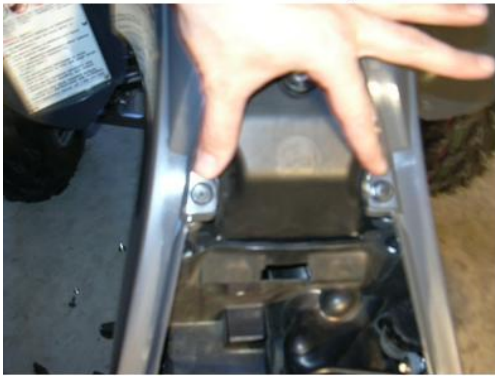
9. Plastic inserts, use fingers to twist out
