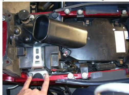
24. 10mm bolts if you want to remove the battery to clean the rubber shielding
