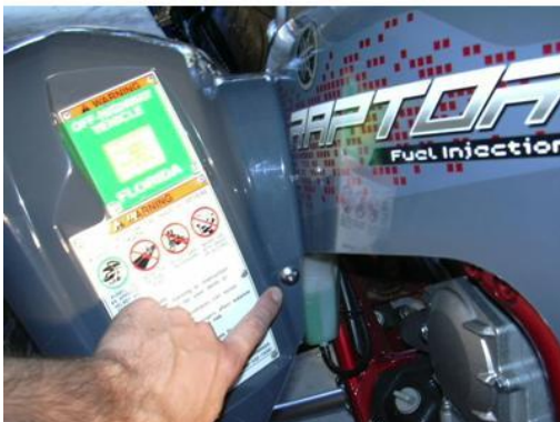
5. 10mm nuts on back of Allen screws
