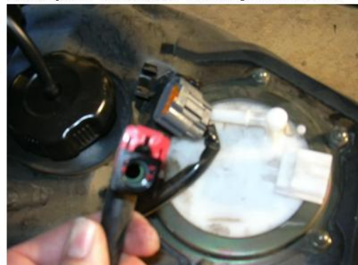
20. Clip removal for fuel line and connections for fuel pump. Take your time, no tools, just hands
