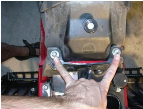
17. 10mm rear gas tank bolts
