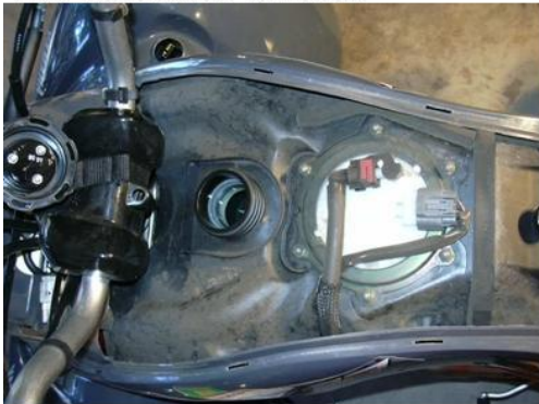
13. Top of gas tank showing connections that need to be removed
