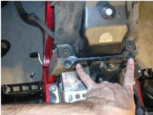
21. Plastic inserts, use fingers to turn 1/4 turn and pull up
