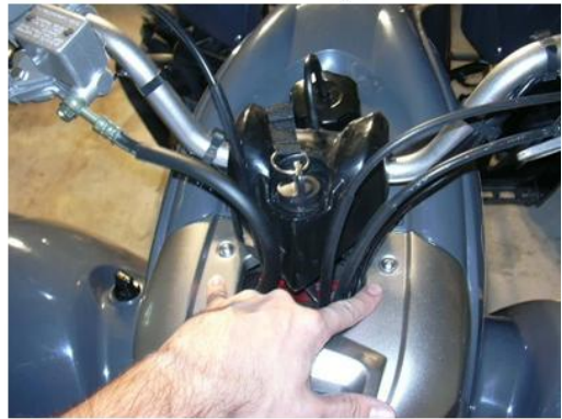
2. The two Allen screws holding the cover on
