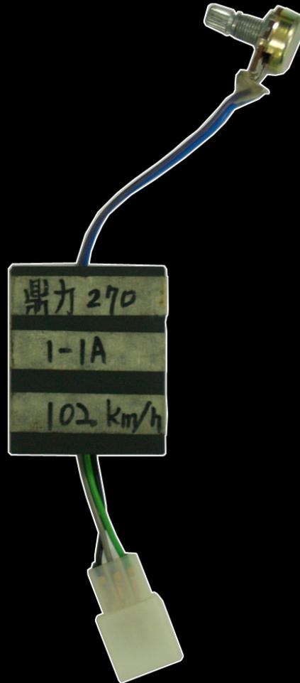
※The shape of your speed simulator could be different than above shows but the functions will be the same.
