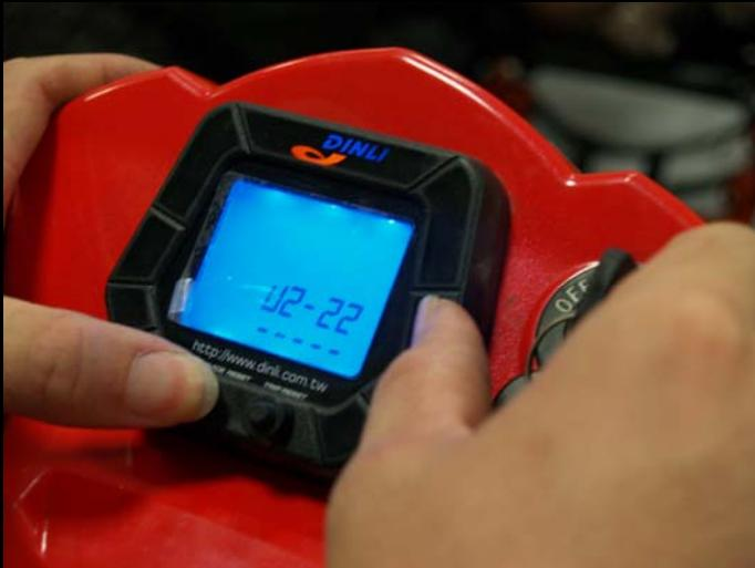
Keep pressing the left key and turn the main switch on.
