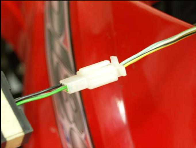
Connect the plug of simulator to speedometer as shows.
