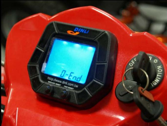
When above screen comes, press the right key then "End" flash, press the left key.
