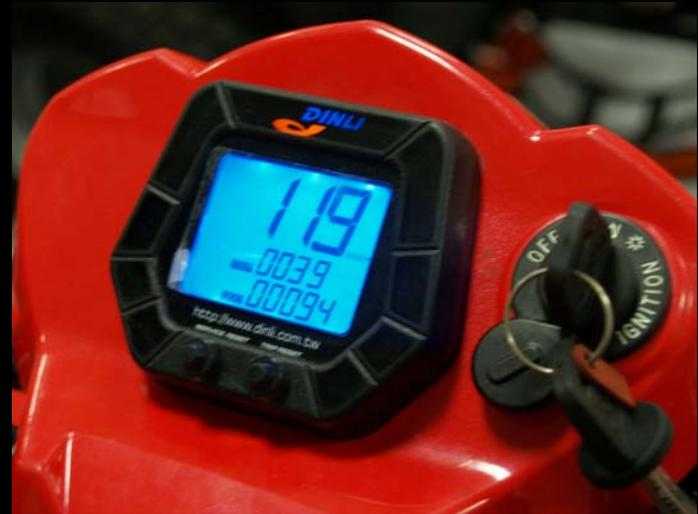
Use the speed simulator to make the speed reach between 115~120km/hr.
