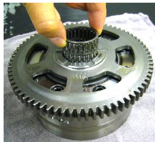
Remove oil from taper portion
