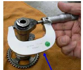
Visual checking for cam profile and Measure the height Micrometer
