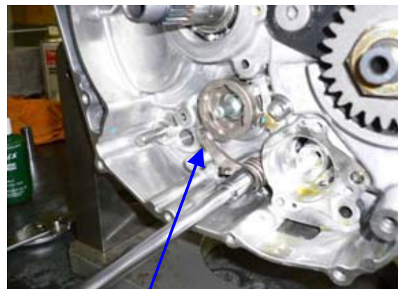
Hook Spring (stopper) into the groove behind Shift C Stopper Arm CP
