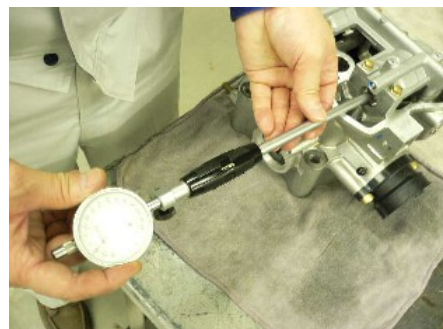
Visual checking for cam profile and Measure the height Micrometer
