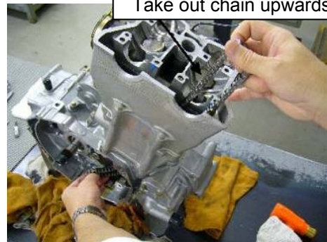
Take out chain upwards
