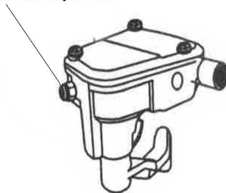
throttle adjust bolt
