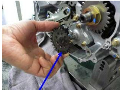
Oil Pump Gear
