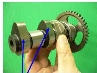
Visual checking for cam profile and Measure the height Micrometer
