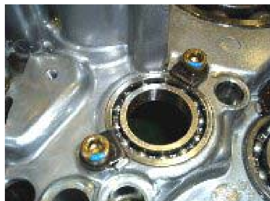
Bearing Retainer Plate B ; 2pcs.
