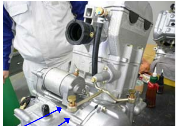
Gasket arranged on both side of Banjo bolt
