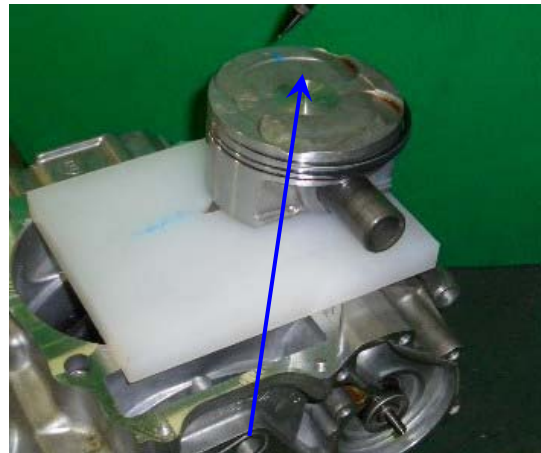
Marking be faced to MAG side
