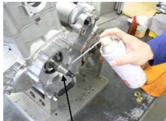
Remove oil from taper portion
